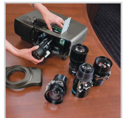
Four optional user-replaceable bayonet lenses—just push, twist and replace.
